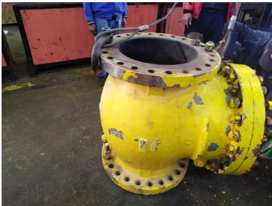
Figure (3-3): Maintenance of the check valve in SIC plant.
