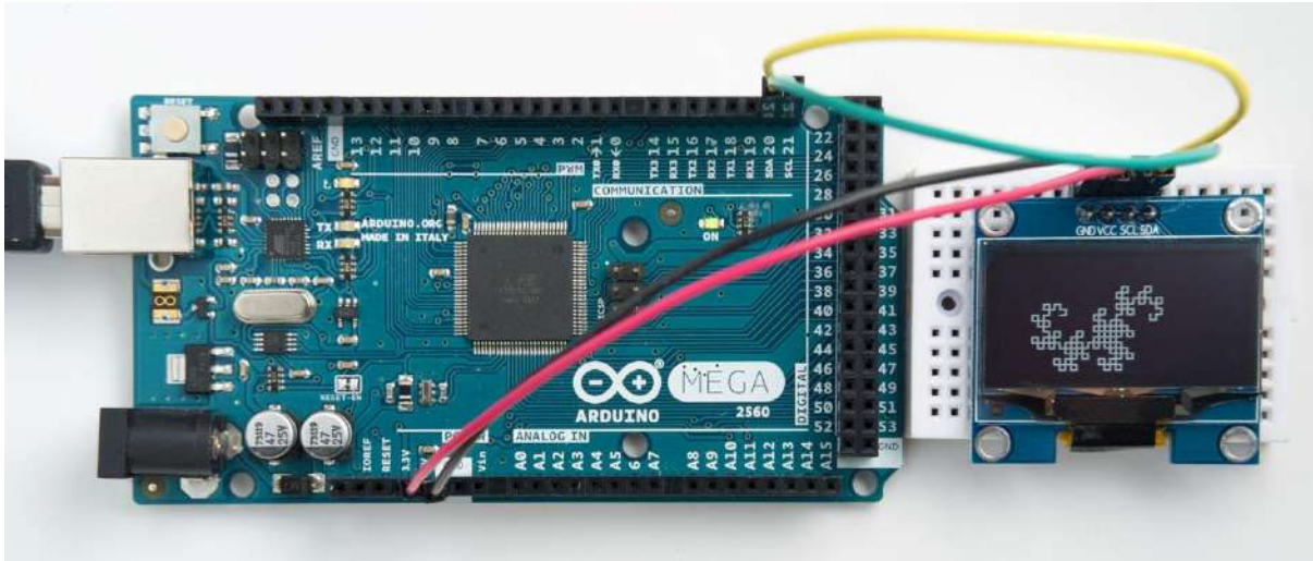
Figure 3-4: OLED DISPLAY CONNECTED WITH ARDUINO
