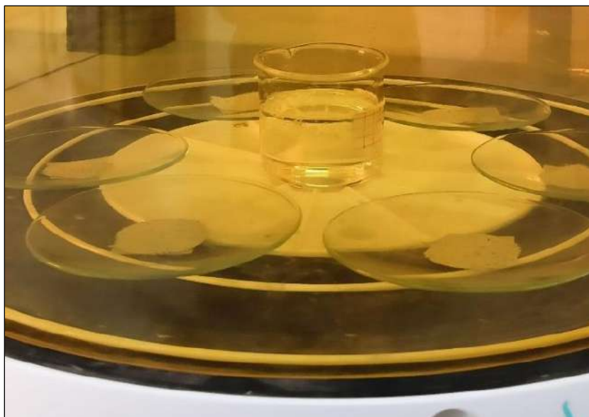
Figure.II.5 Acidity analysis of zeolites using the gravimetric method for pyridine adsorption
