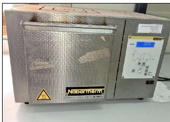
Figure .II.4 The dried mass finally has to be calcined at 450°C for 2 hours precededstages of 1 hour at 150°C, 250°C and 350°C.
