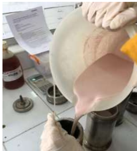
Figure II. 7: Filling the Ageing Cells with Drilling Fluid.
