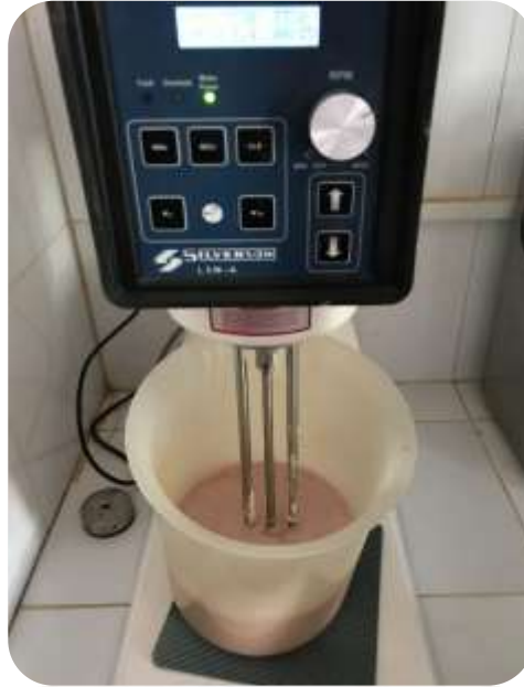
Figure II. 1: Mixing the HydraGlyde Mud.
