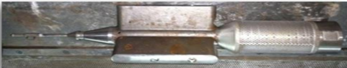
Figure 46 : control shaft control shaft lubrication and filter [37]
