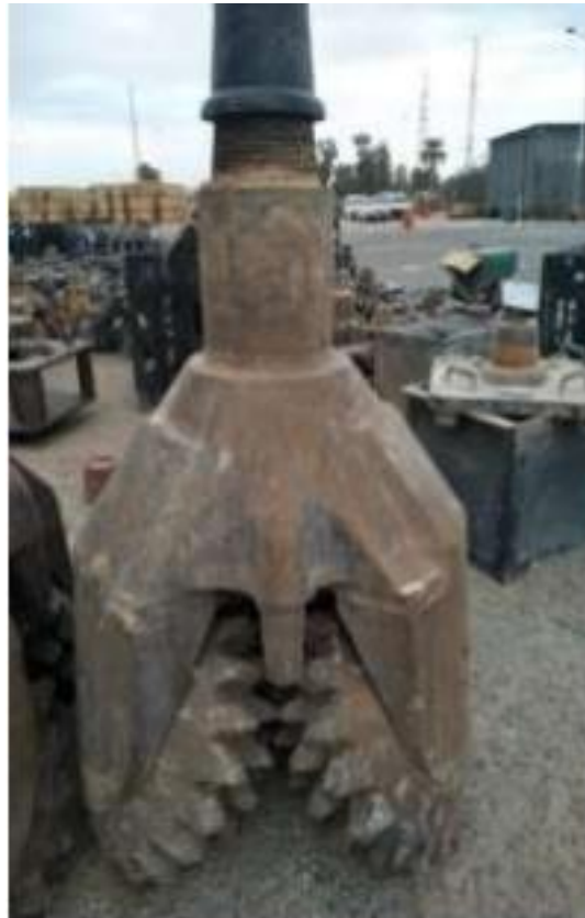
Figure I.6: outil tricône réelle
