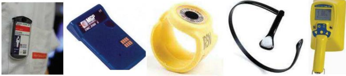
Figure II-8: Examples of measuring devices (in order: chest passive dosimeter, chest operational dosimeter, ring passive dosimeter, crystalline passive dosimeter, contaminometer) [48].
