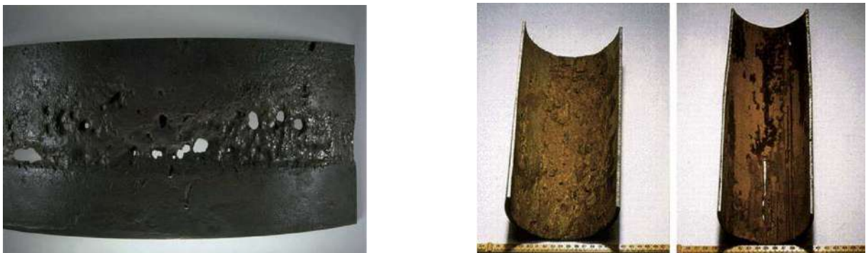
Figure I-3: Images of Localized corrosion [2].
