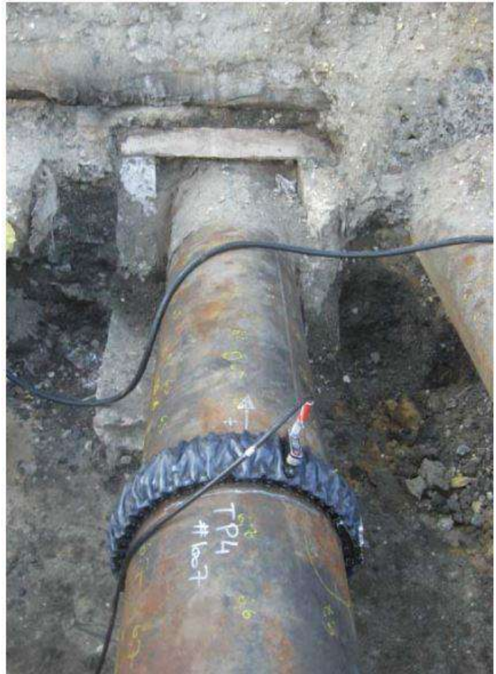
Figure III-10: Flexible ring for pipe inspection
