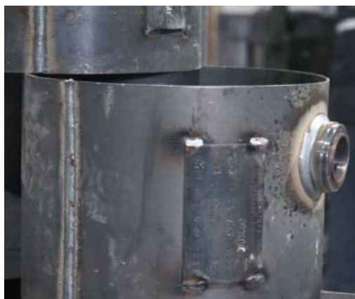
Figure II.6: Cylindrical tanks under manufacturing [16].
