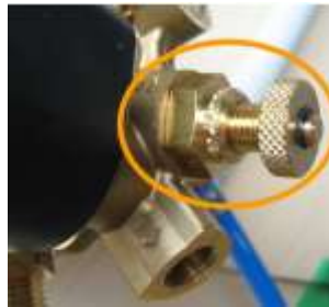
Figure II.13: The manual valve [20].
