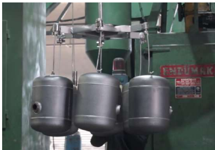
Figure II.8: Coating the tanks [16].
