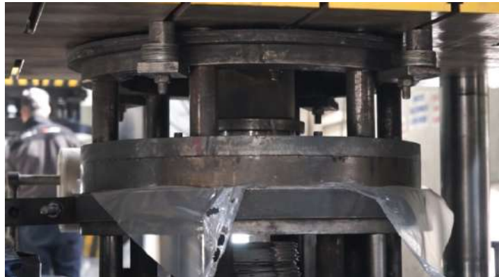
Figure II.5: Forming a half-tank by means of a pressing machine [16].
