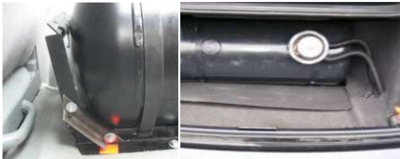
Figure II.2: A fitted LPG tank [12].
