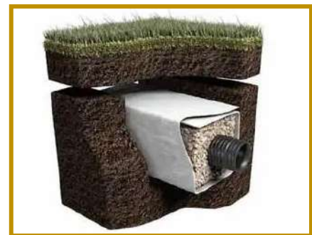
Figure 1.10: Geotextiles for drainage.
