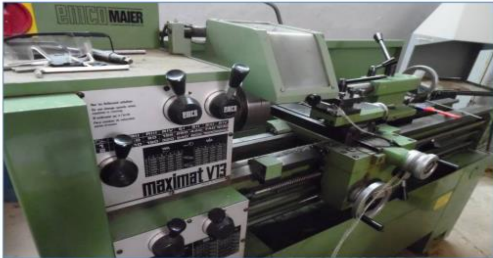
Figure II. 3: Tour parallèle universel
