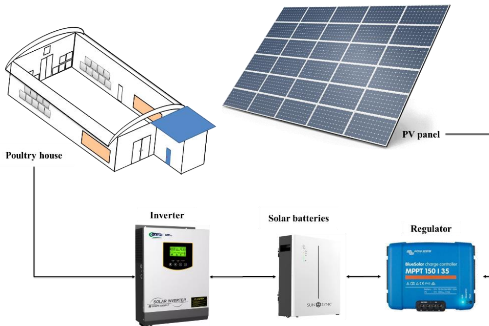
Figure III-9: photovoltaic system Component
