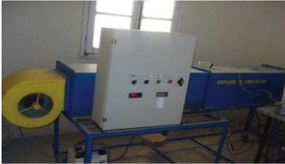
Fig II.3. Laboratory-scale convective air dryer of INAT [25]
