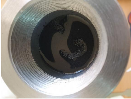
Figure III. 22: Placing the proppant sample and fracturing fluid in the containment cell
