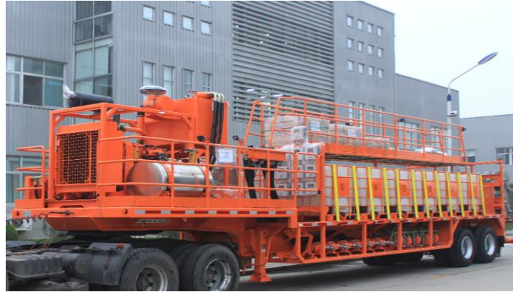
Figure I. 19: Chemical additive unit [22]
