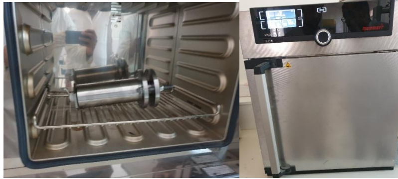
Figure III. 24: Placing the sample in the oven
