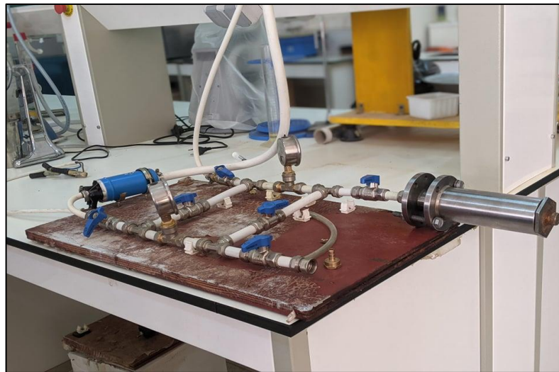
Figure III. 14: Schematic diagram of proppant permeability measurement system
