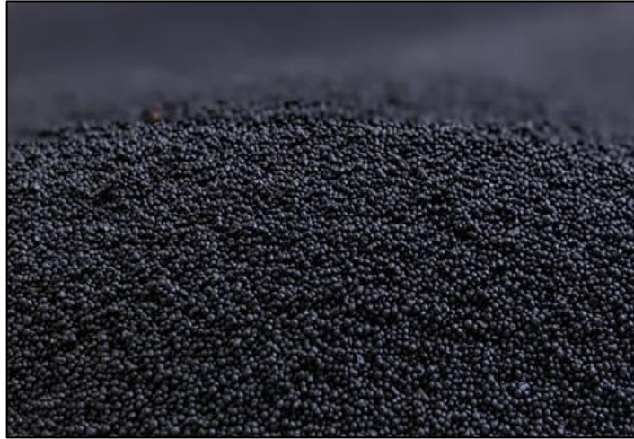
Figure III. 6: Bauxite proppant of size 20/40 used in the experiments [26]
