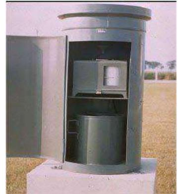
**Figure II.9 : Pluviographes source (IHFR)**
