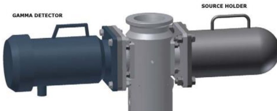
Figure 22: Gamma source and detector make up the gamma densitometer[9]
