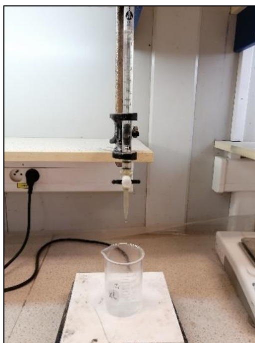
Figure III.7: Acid-base titration instrument. [32]
