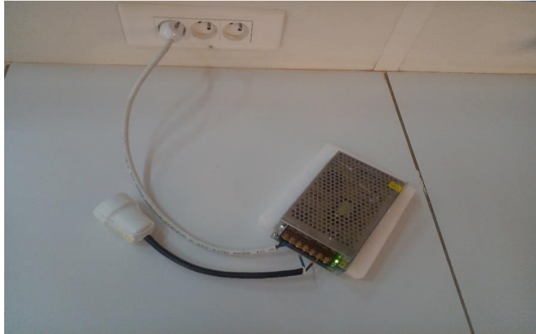
Figure I.9: A 9-12V SCR unit used for experiments.
