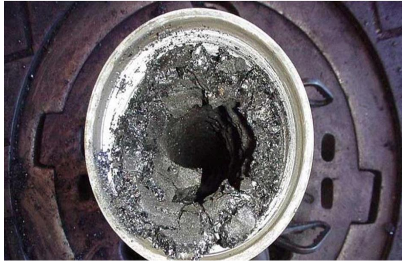
Figure I.A.6: asphaltene disposition inside tubing [11]
