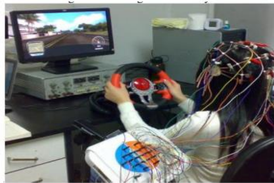
Figure 5 : EEG data acquisition system.
