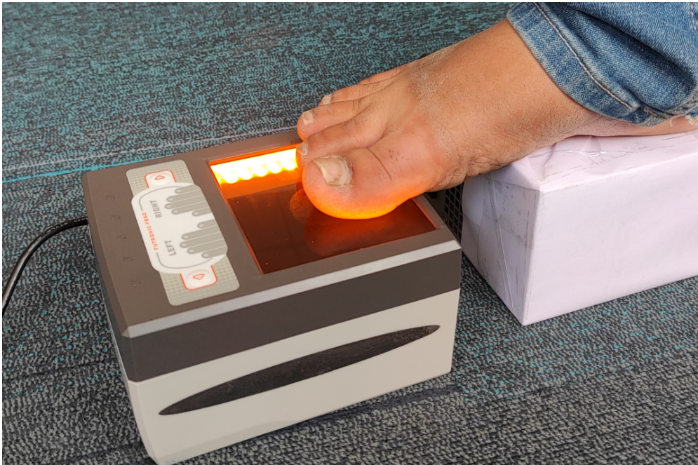
Figure 2.27: Acquisition of toe print using Futronic FS60 optical fingerprint sensor
