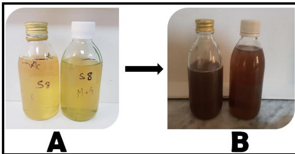
Figure 9: A: culture supernatant with AgNO 3 solution (no color change) B: culture supernatant with AgNO 3 solution after synthesis (with color change)
