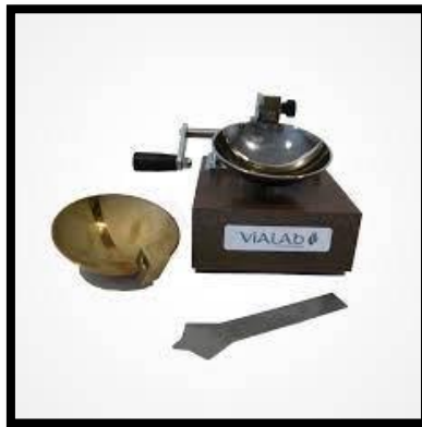
Figure II.5:Appareil de Casagrande
