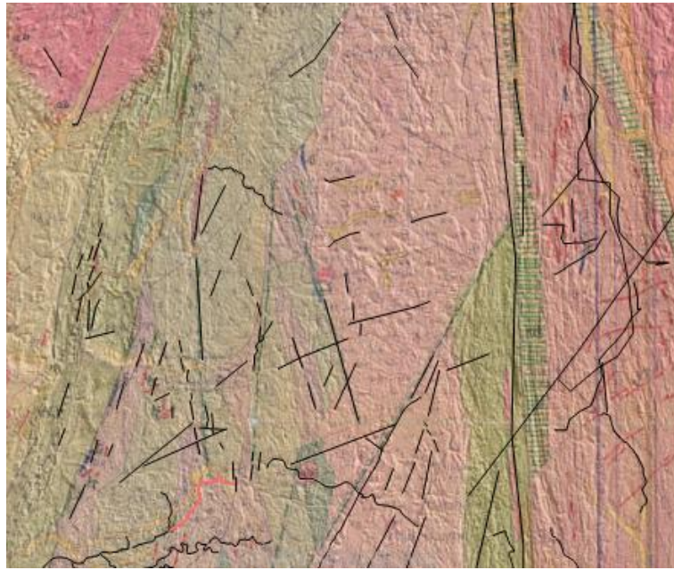
. Figure: extraction Map of the lineaments using DF 135° M 7x7 and geological map
