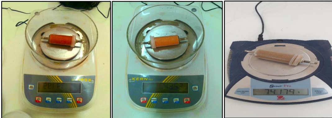
Figure III.5: weighing the wet sand sample, saturated sand sample and asphaltene sand sample respectively
