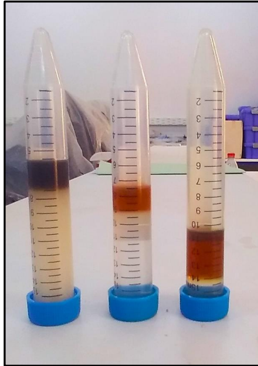
Figure IV.14: samples of the recovered oil after brine flooding, nanosilica flooding and nanosilica flooding with polymer injection respectively from right to left.
