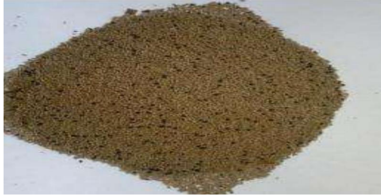
Figure I.8: Intermediate strength Proppant [12]
