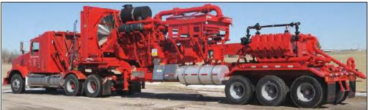
Figure I.18: High pressure pumps.[19]
