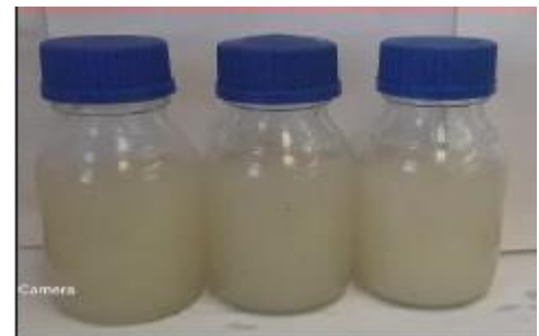
Figure III.10: MiniFrac Cross-linked Gel
