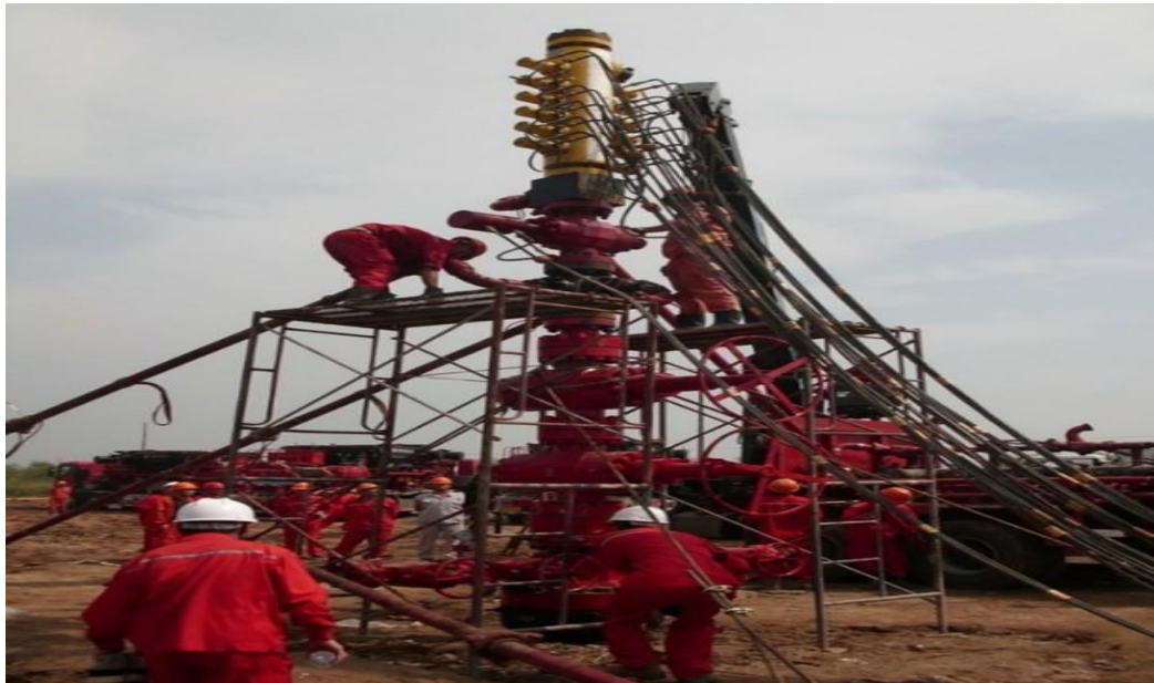
Figure I.19: Wellhead isolation tool.[19]
