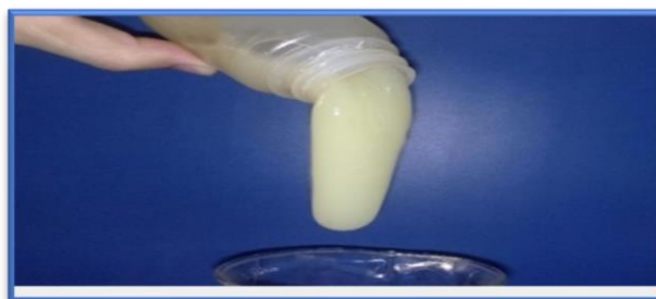
Figure I- 4 A sample of water-based fracturing fluid [2]
