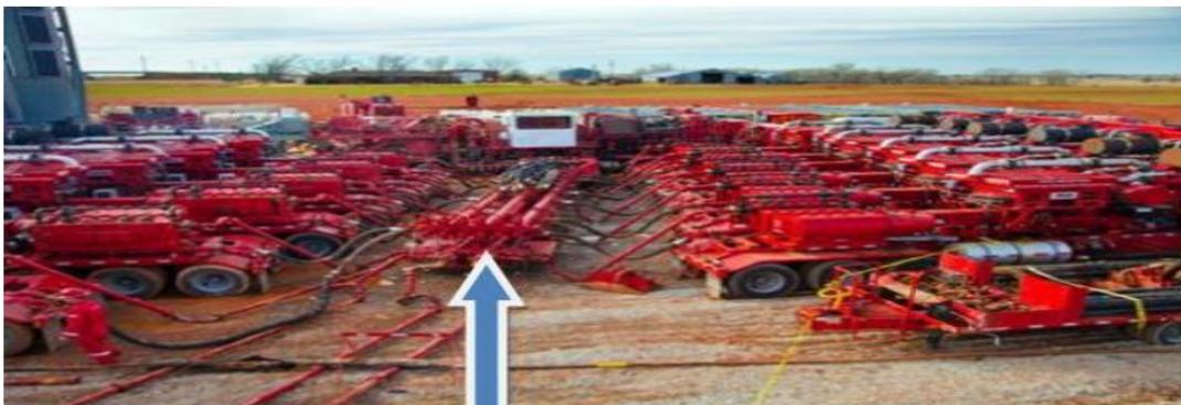
**Fig II-26 :** Manifold de haute pression.
