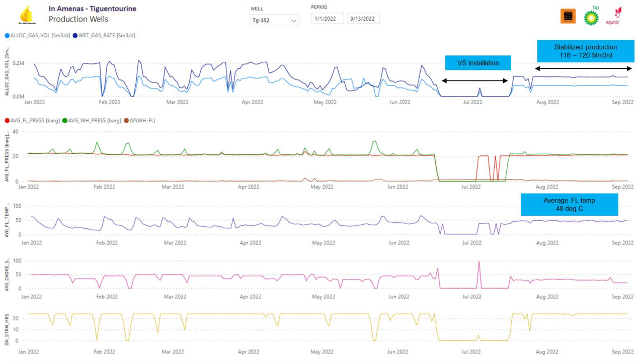
FIGURE 62: PRODUCTION OF TG-362 BEFORE AND AFTER VC INSTALLATION
