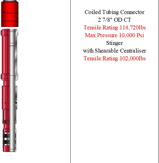
FIGURE 76:STINGER BHA SCHEMATIC
