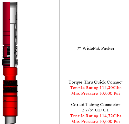
FIGURE 77: WIDEPACK HANGED BHA SCHEMATIC
