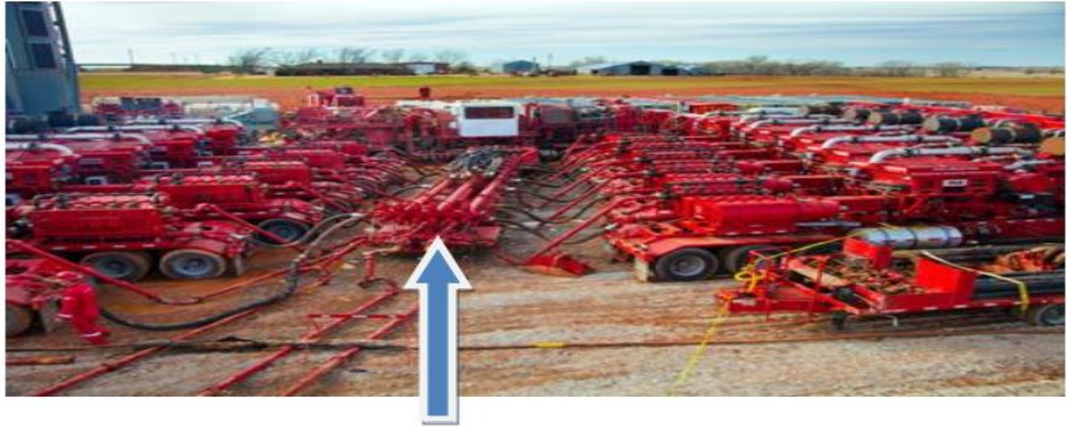
Fig.III.7 Manifold de haute pression
