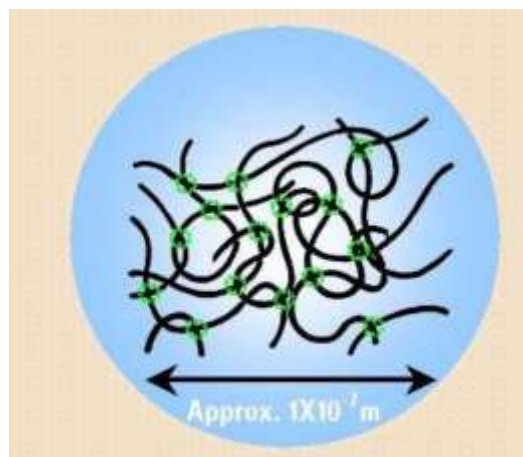
Figure 3- 20 An Illustration of the Cross Linked Fluid on the Microscopic Level [21]
