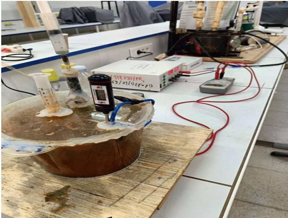
Figure I- 8: Typical electrolyser utilize in experiment.
