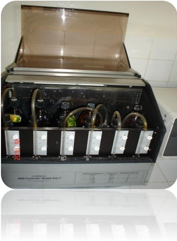
Photo Appareil \text{DBO}_5 (Mf 120)
