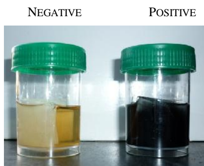
Figure 1. The illustration of the results interpretation of the hydrogen-sulphide test kit.
