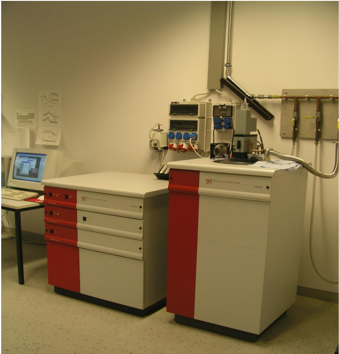
Fig.3.2: superconducting quantum interference device (SQUID) magnetometer “MPMS 5” from Quantum Design Experimental Physics V, Centre for Electronic Correlations and Magnetism, Institute of Physics, University of Augsburg, 86135 Augsburg, Germany.
