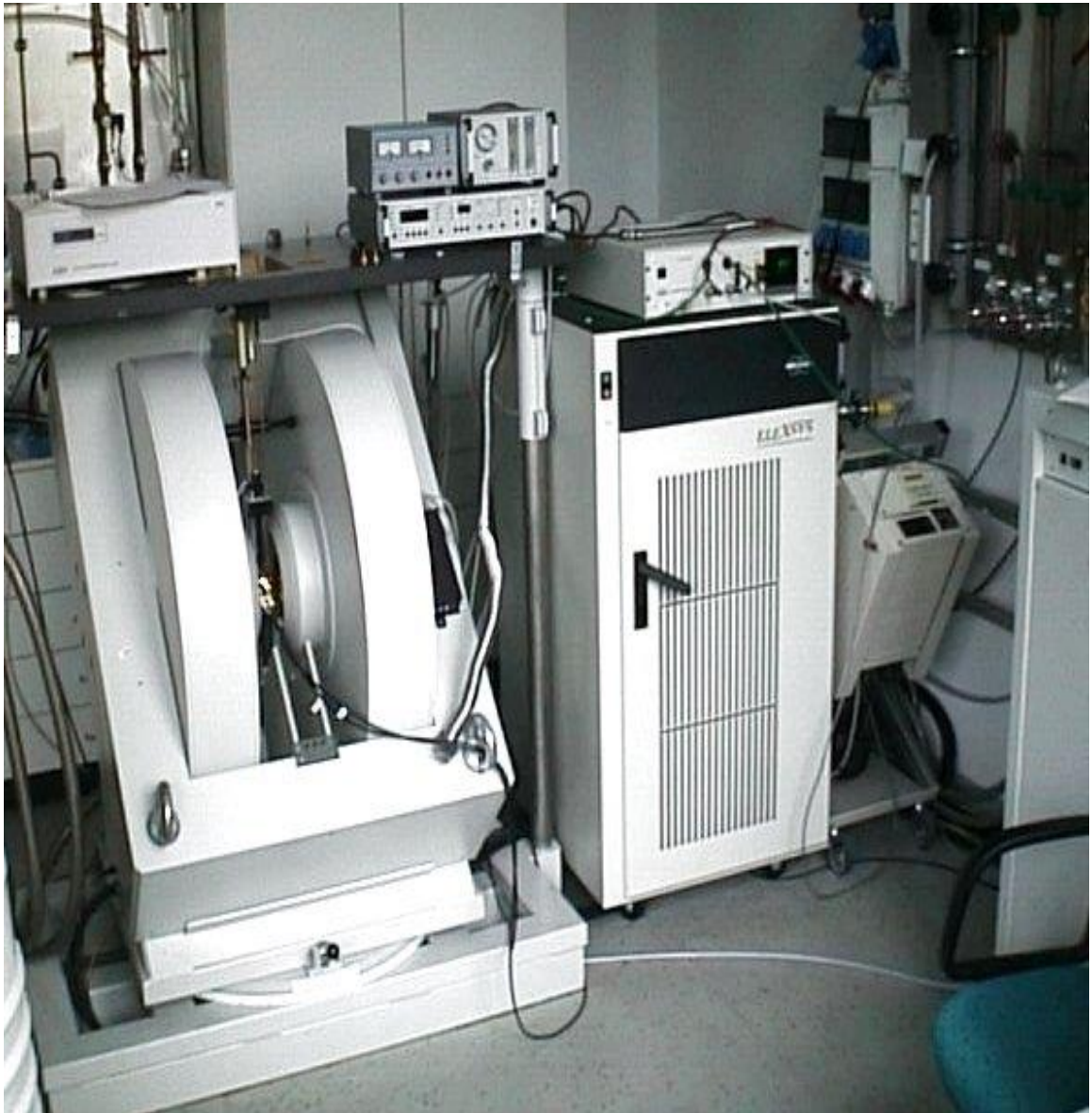
Fig.3.3.: ESR-Spektrometer Bruker ELEXSYS E500-CW Experimental Physics V, Centre for Electronic Correlations and Magnetism, Institute of Physics, University of Augsburg, 86135 Augsburg, Germany.
