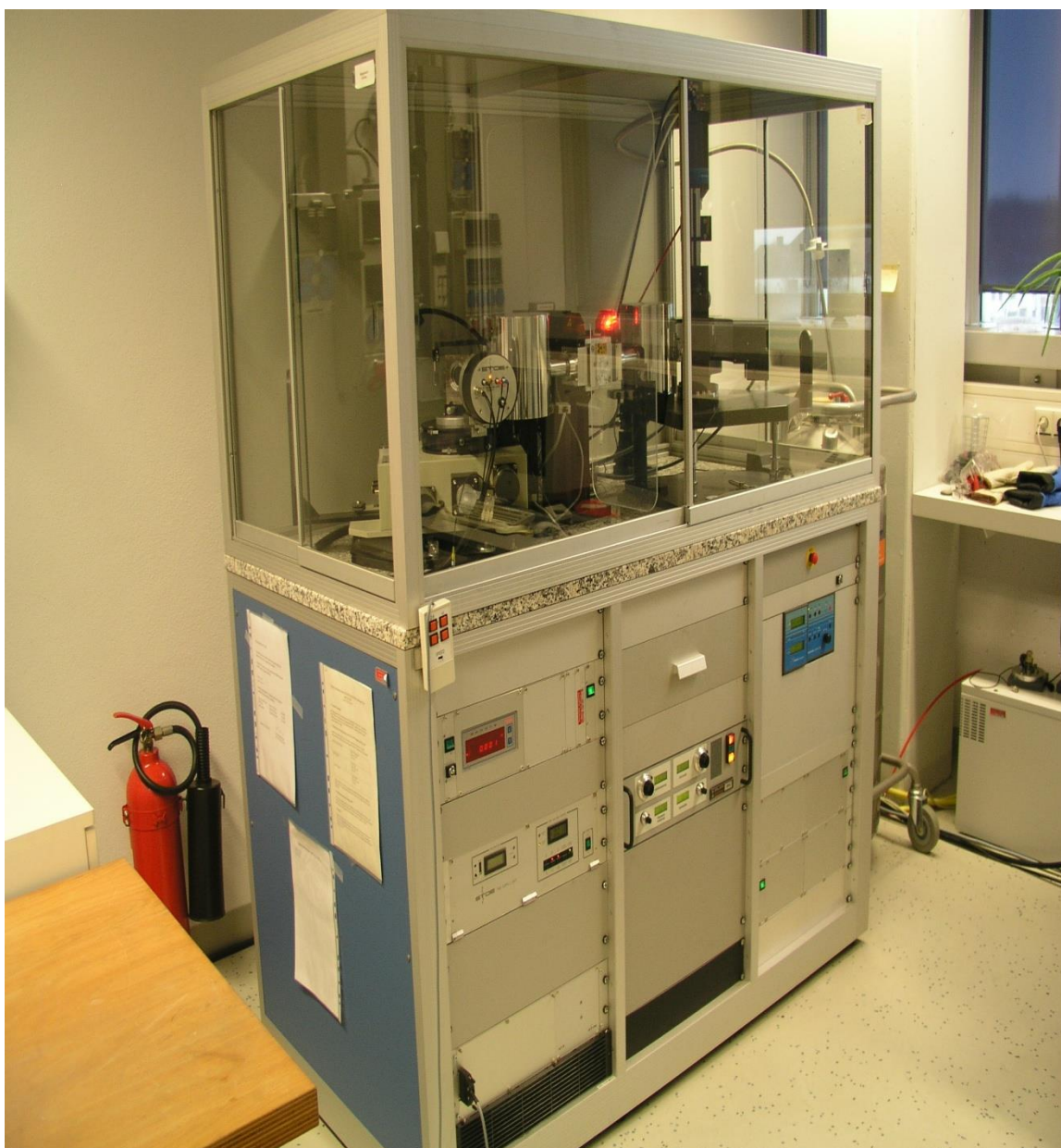
Fig.3.1: STOE STAD-IP diffractometer , Experimental Physics V, Centre for Electronic Correlations and Magnetism, Institute of Physics, University of Augsburg, 86135 Augsburg, Germany.
