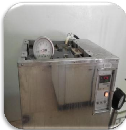
Figure III.11: Mesure de la TVR
