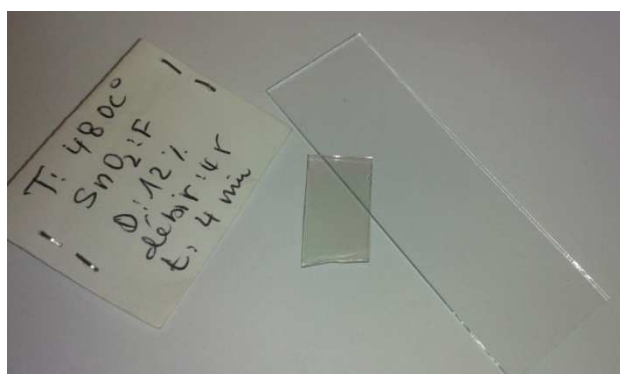
Figure III.4: Glass coated by F doped SnO 2 thin film.
