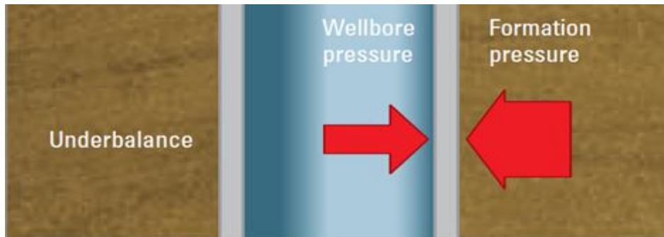
Fig III-7 : Perforation en underbalance
