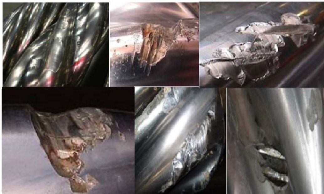
Figure (III.15): Rainurage (coating & base material gouging) de rotor.
