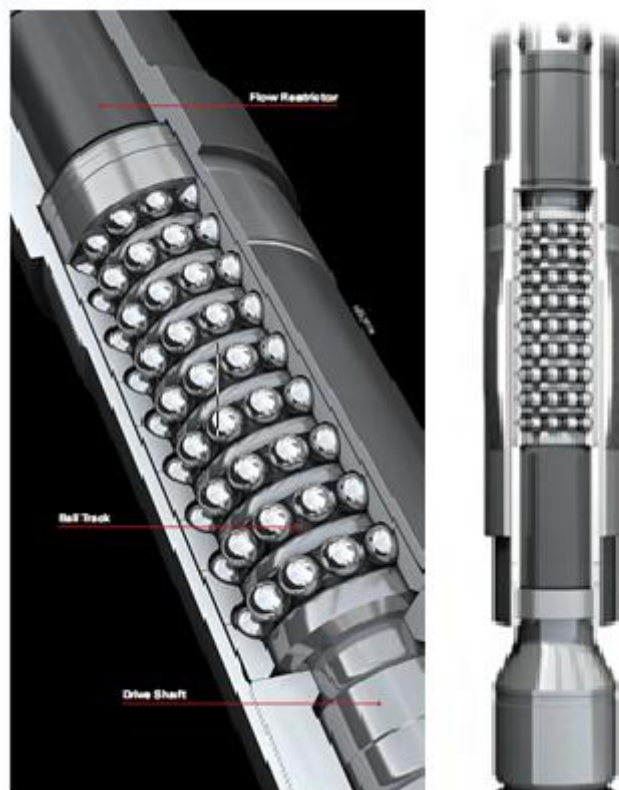
Figure (I.2) [3]: La section de roulement.
