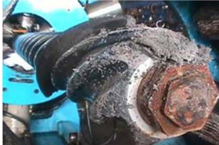
Figure (III.16) : La contamination de rotor.
