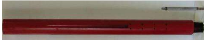
Figure 23 Downhole Air Diverter (DHAD) 26
