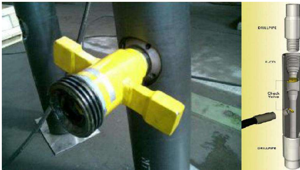
Figure 28 Continuous Circulation Valve (CCV) 24
