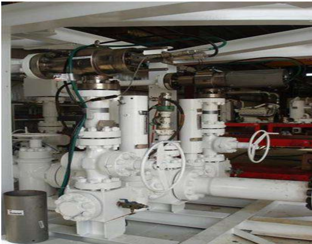
Figure 18 Semi-Automatic Choke Manifold System 26
