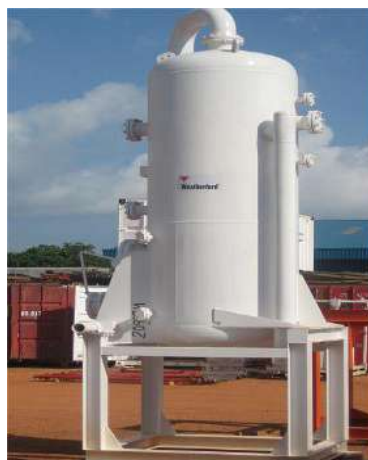
Figure.I.12: Separator in Weatherford Company.
