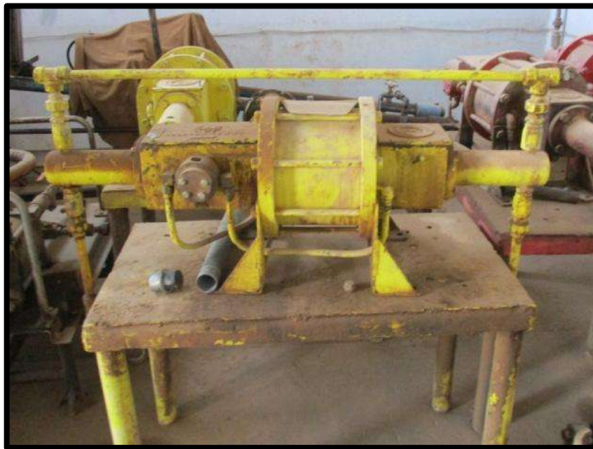
Figure III.3 : la pompe BSB
