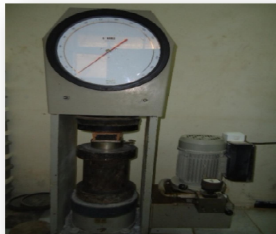
Photo III.6 : Essai de compression
