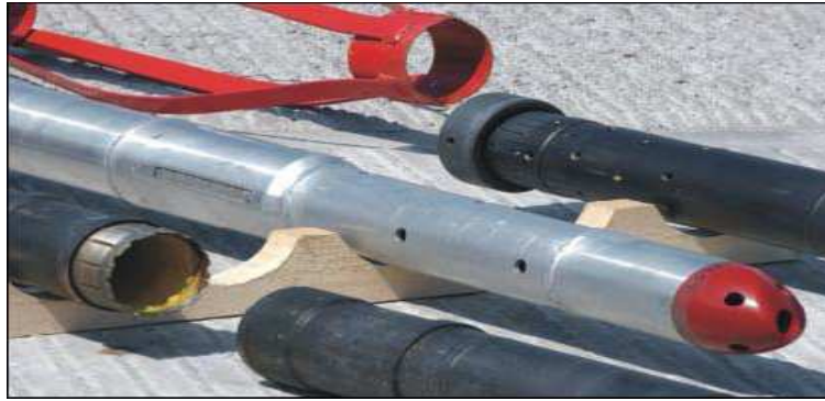
Figure IV.4: Composantes de l'expandable casing.
