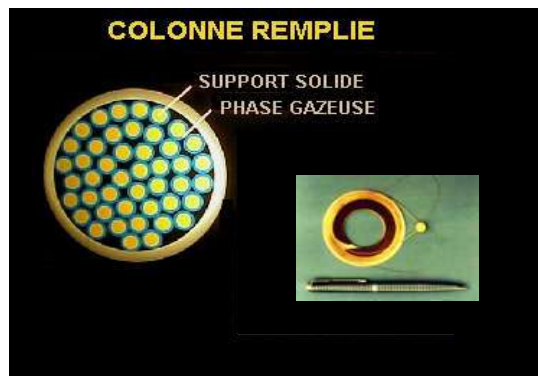
Figure 2.16 colonne de gaz
