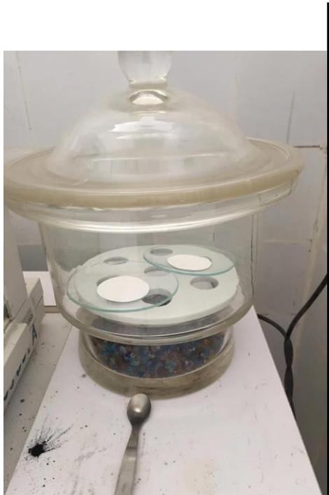
**Figure (III-11) : Dessiccateur**
