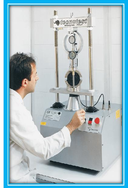
**Photo II.2 Application de la compression Marshall**
