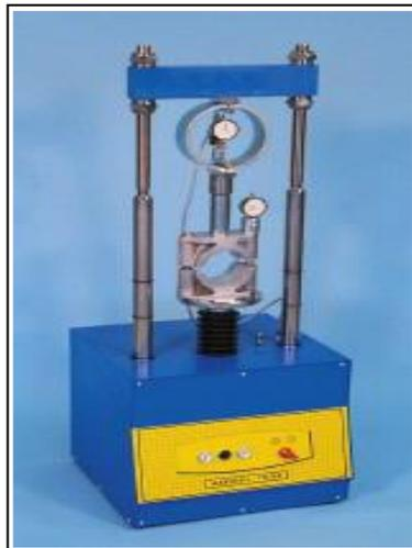
**Figure I.21. Presse de compression Marshall**
