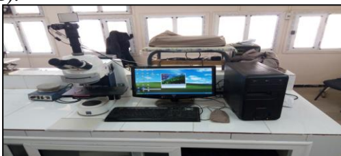
Figure V.1: Microscope optique, objectives: 5X, 10X, 20X.
