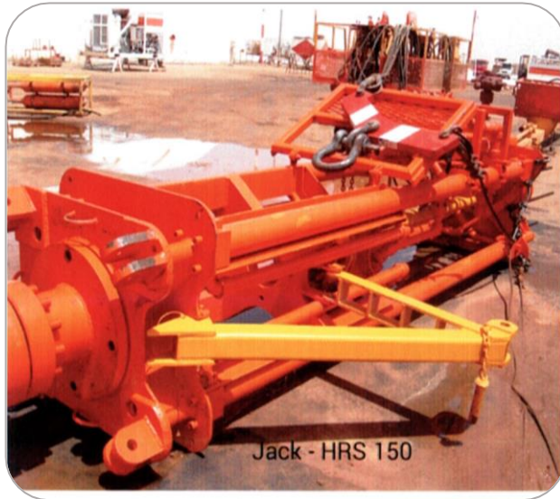
Figure 13 : Ensemble de vérins hydrauliques (Hydraulic Jack Assembly)
